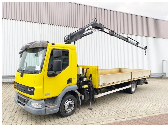
DAF AE 45 LF 220 4x2, Kran MKG HLK 71 HP A 3, Funk
